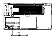
Note: Before installing the next set of batteries, verify that the frequency step selector switch is set to the position correct for your country. In the USA, move the swifch to the 10K position. In other countries, set it to 9K.
